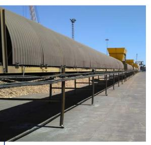
Figure 3. Example of permanent facilities at a similar port, with hoppers close to ship holds and fixed conveyor belts.
